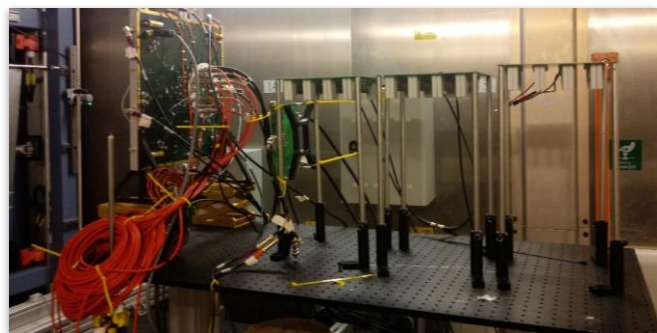
Fig. 7. Test boards setup for the first campaign under neutron beam at ISIS ChipIR facility. The beam output is on the left side of the picture. DUTs in this work are positioned on the first and third board from the left.
